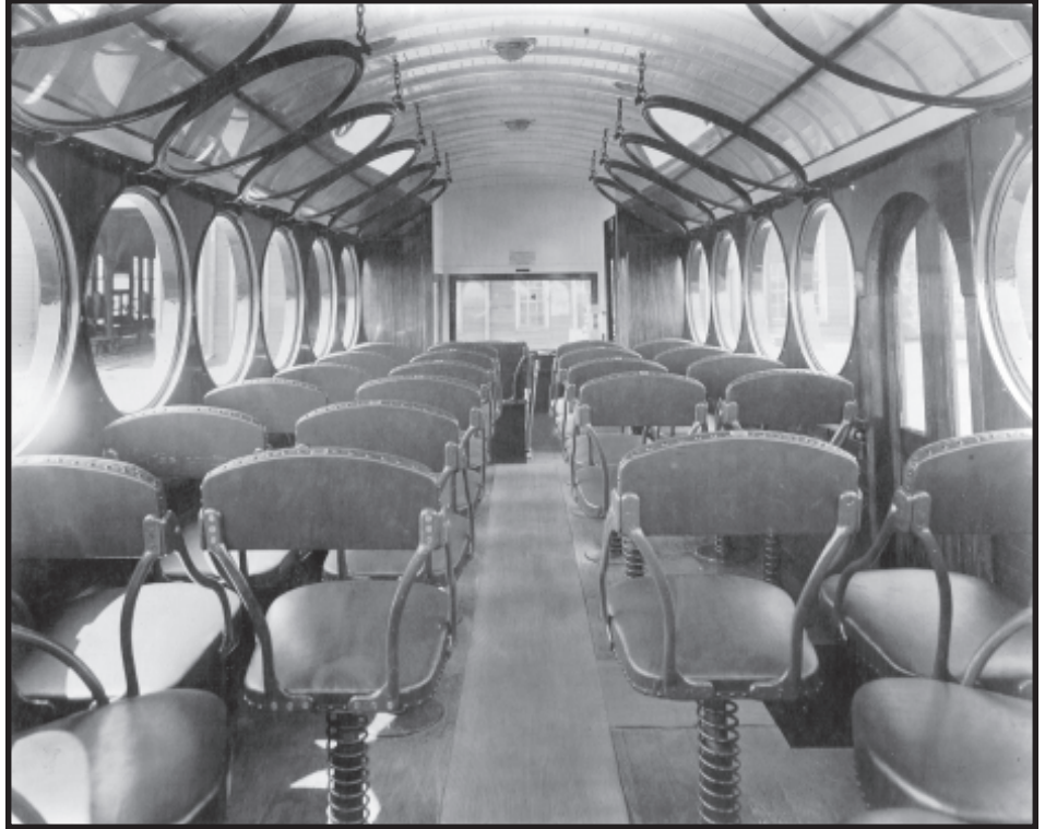
Interior of the McKeen chair car. Note the unusual suspension. Photo from the George N. Andrews Collection. NSRM
