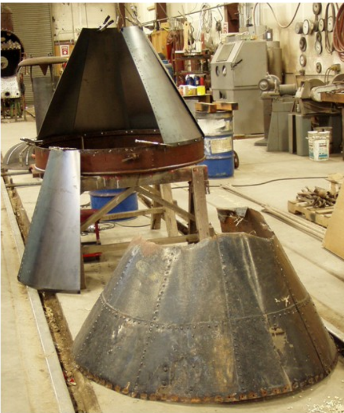
The original stack sits below its replacement. January 2012
