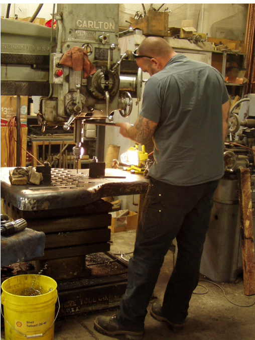
Restoration Specialist Mort Dolan, drilling 2" diameter holes in the rear tube sheet for the new boiler tubes. January 2012
