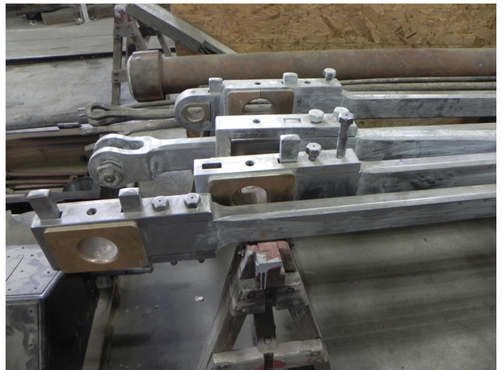
The rods have been fitted with new brasses and bolts. January 2012
