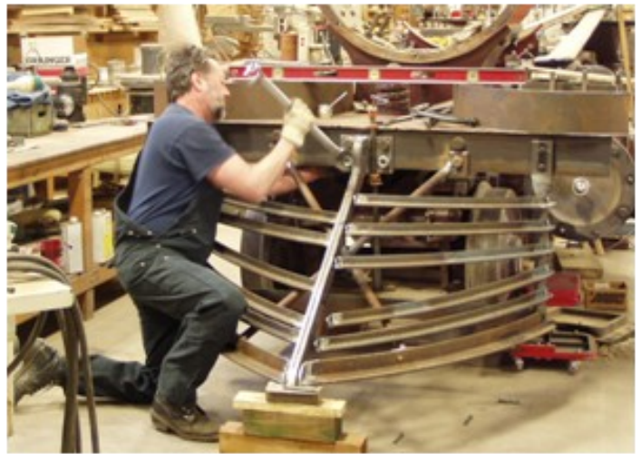
Restoration Specialist Rick Stiver fabricates the new pilot. February 2012
