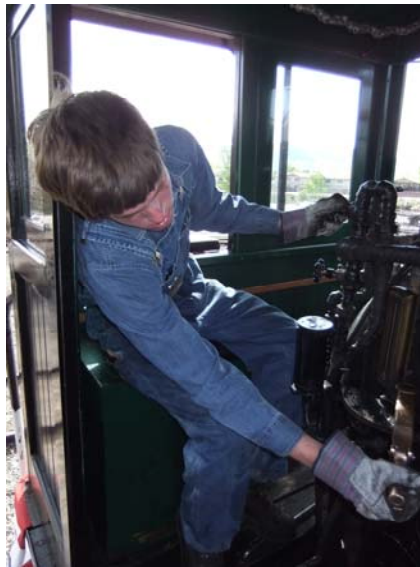
With atomizer (in left hand) and firing valve (rt.) Volunteer Kevin Owens regulates fuel-oil flow.
