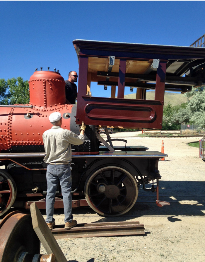
Curator of History Wendell Huffman (bottom) and Restoration Specialist Mort Dolan assist Restoration Specialist Rick Stiver (not pictured) place the cab on the Glenbrook on June 30, 2014. NSRM Photo.
