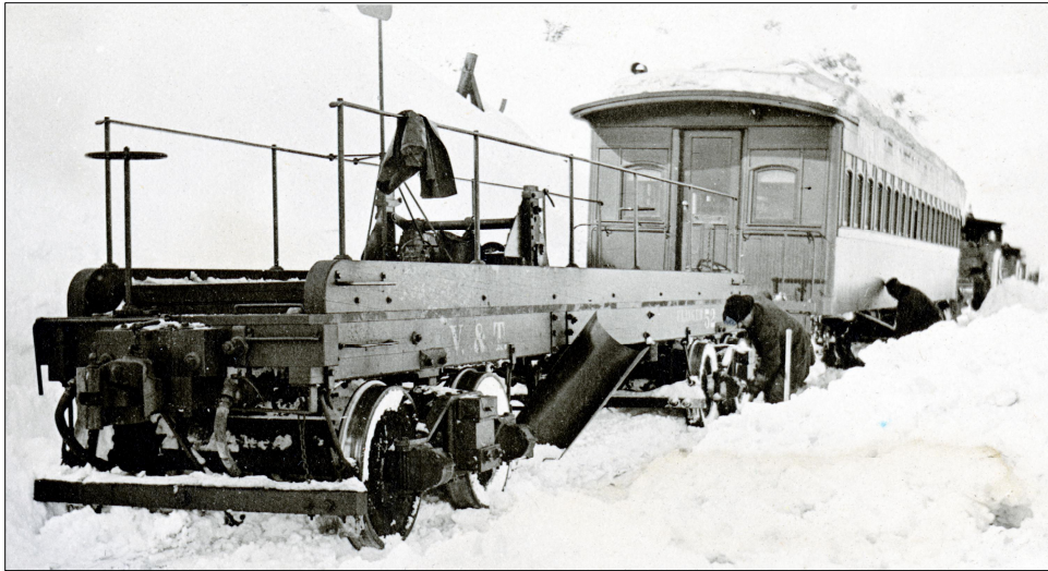
The V&T flanger goes off the rails with Coach 17 during a snowstorm in Carson City, January 1916. V&T No. 25, Coach 17, and the flanger had a unique air system tying them together for plow train service. Photo: University of Nevada, Reno, Special Collections Department.
